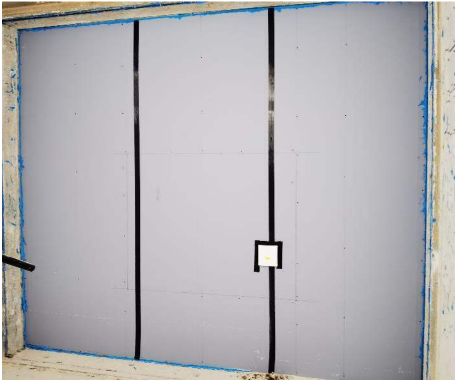
Photograph 2: SODAC passive wall ventilation, internal grill surface mounted (Receive room).
