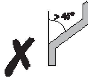
Ducts should use no more than one offset (i.e. no more than two bends) and these should be of the “swept” rather than “sharp” type to minimize flow resistance. Offsets at an angle should be no more than 45° to the vertical (Diagram 3).
