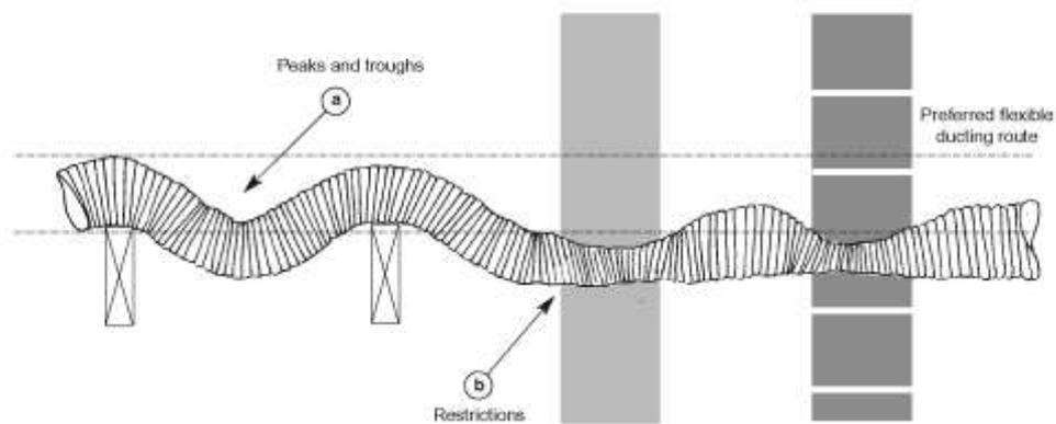
The inner radius of any bend should be greater or equal to the diameter of the ducting being used. If the radius is reduced, the resistance of the bend will increase and the volume of air being extracted will decrease (see “Do” Diagram). Ensure flexible ducting is installed without peaks or troughs (see “Don’t” Diagram).
