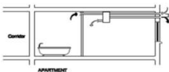
**Diagram 2c: Natural Ventilation with intermittent fans mechanical extract - House**
