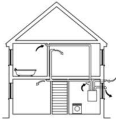
**Diagram 2b: Mechanical ventilation with heat recovery – Apartment**
