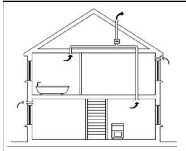
**Diagram 1b: Continuous Mechanical Extract Ventilation - Apartment**
