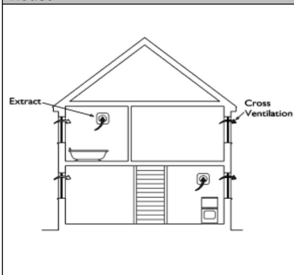
**1.2.1.5** Where both open flued combustion appliances (including open fires) and extract fans are installed in the same
