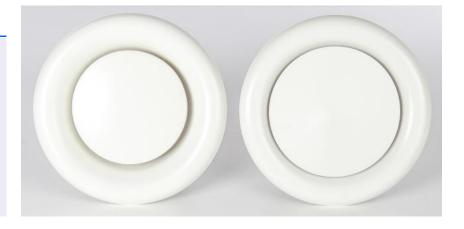
The FIREFLY Fire Rated Ceiling Air Valves are a unique and cost effective fire rated solution where recessed ceiling air valves are to be installed in fire rated ceilings. In a fire situation, the integral intumescent material rapidly expands to seal off the air valve and reinstate the fire resistance rating of the ceiling. This limits the risk of fire and heat spread throughout the building. The Ceiling Air Valves are available in all sizes for both Extract and Supply.
